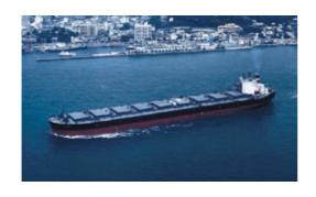
the work horses of the fleet, these transport raw materials such as iron ore and coal. Identifiable by the hatches raised above deck level which cover the large cargo holds.
